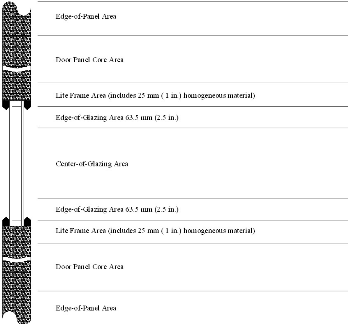
Figure 5-11 Garage Door 2: Vertical Elevation, Glazing Area
