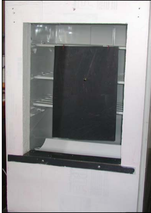
Figure 36. Thermal Transmittance Apparatus with the Surround Panel and Specimen Opening in Place.
