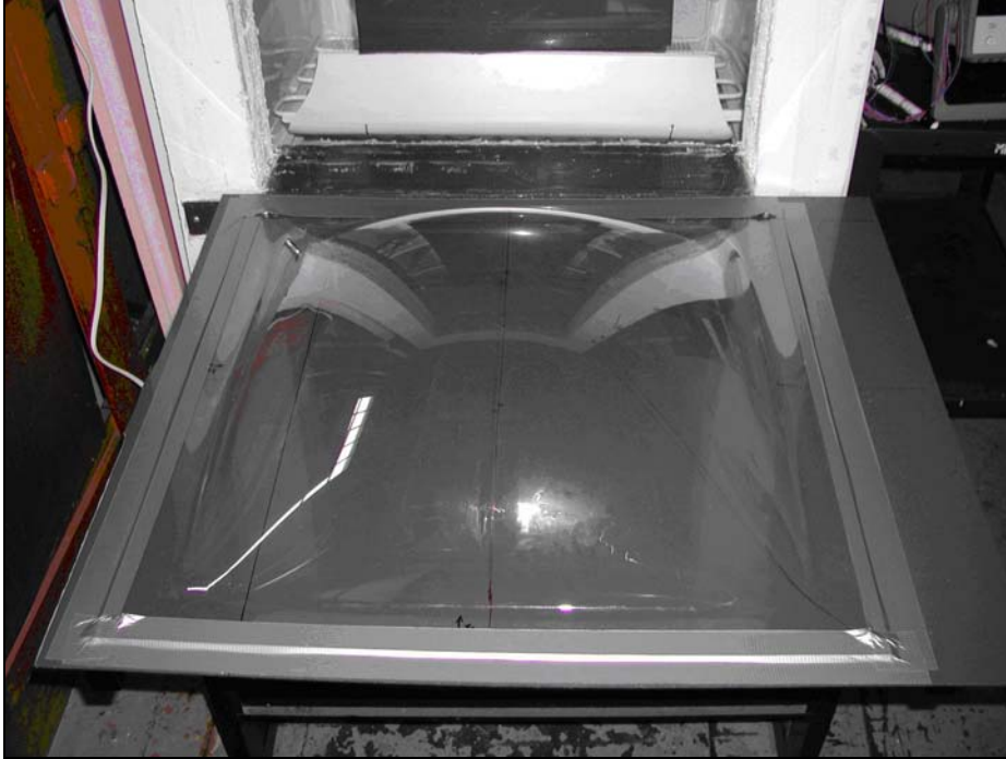
Figure 47. Test Sample for the Type-B Domed Skylight Glazing.
