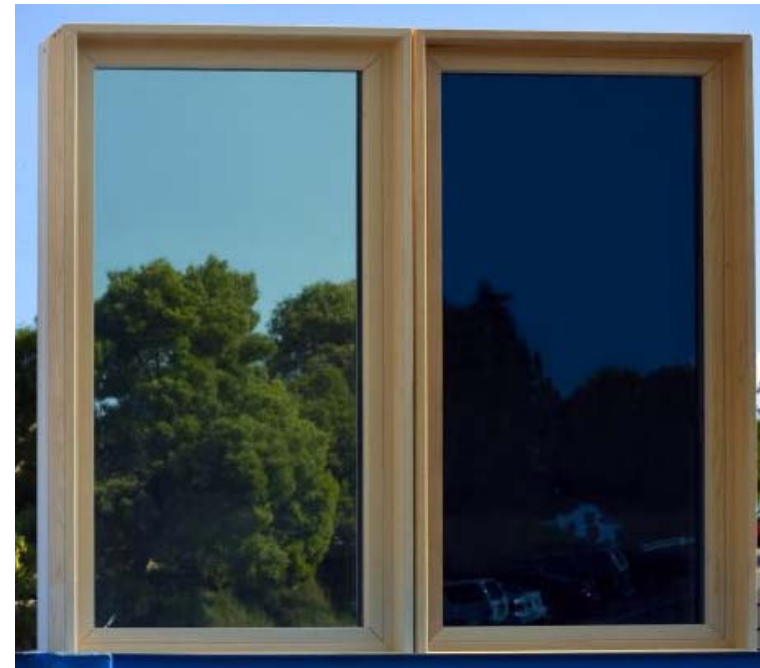
Prototype – Concept Window (Highly Insulating and Dynamic U Value 0.18 (SI U value 1.0) SHGC 0.04 – 0.34) Low cost unsealed center lite
