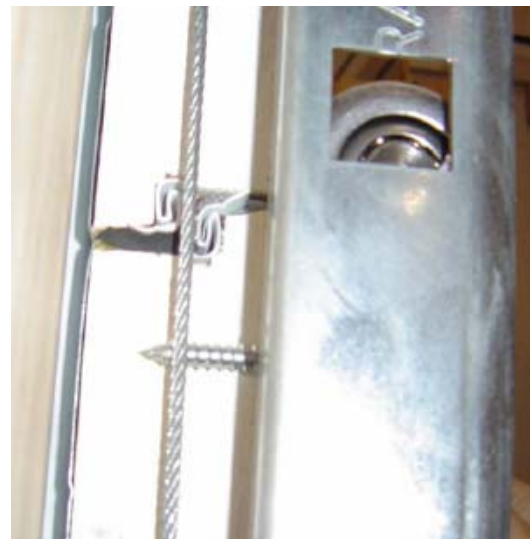
Figure 13 Edge view of Specimen #2 shows thermal break and weather seal (exterior is on the left in this figure)
