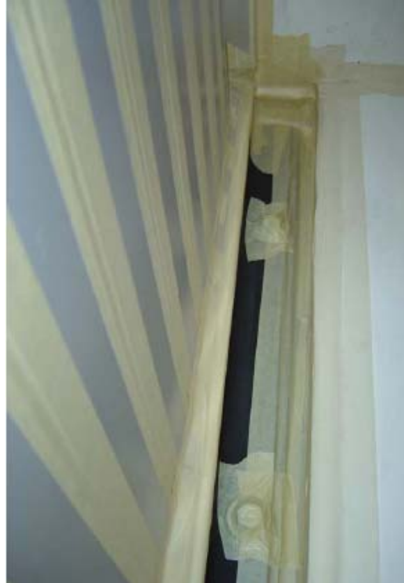
Figure 24 Exterior View of Specimen #5 (sealed before U-factor test to prevent air leakage)
