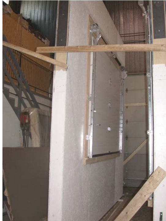
Figure 12 Specimen #2 Insulated Sectional Garage Door (in mask wall)
