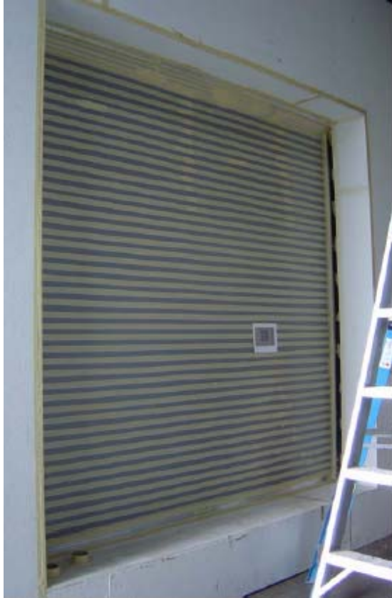
Figure 24 Exterior View of Specimen #5 (sealed before U-factor test to prevent air leakage)
