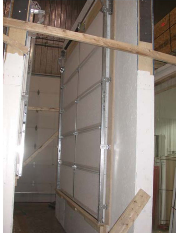
Figure 10 Specimen #1 Non-insulated Sectional Garage Door (rigid insulation in door panels was removed before test)
