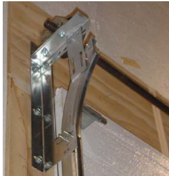
Figure 11 Door track cut to fit assembly into test chamber (for Specimen #1 and #2)
